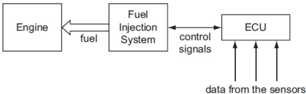
(d) The fuel injection system operates in real time.
