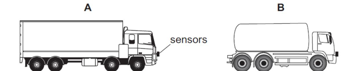
If vehicle A gets too close to vehicle B, the brakes are automatically applied by a computer system in vehicle A.
