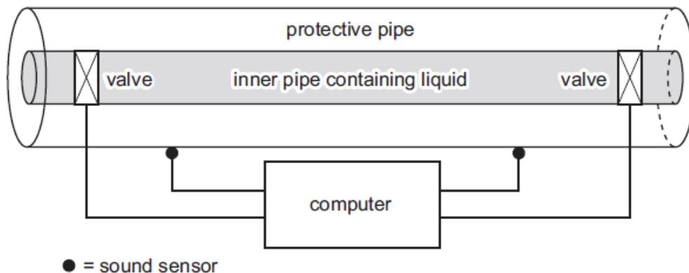
Sensors are used to detect the sound of any liquid dripping into the protective pipe. Actuators operate the valves that regulate the flow of liquid through the inner pipe. This system is controlled by a computer.
