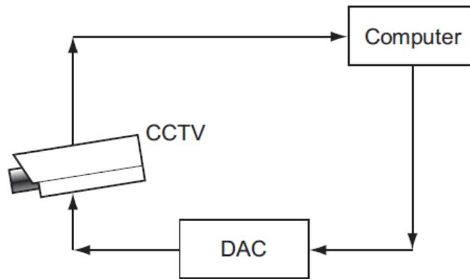
The digital CCTV camera is connected to a computer. The computer can make the camera move in any direction by sending out digital signals. The computer system has a 400 gigabyte hard disk.
