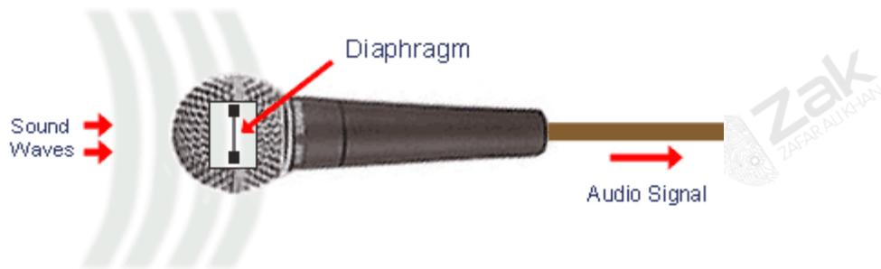
When the diaphragm vibrates, it causes other components in the microphone to vibrate. These vibrations are converted into an electrical current which becomes the audio signal.
