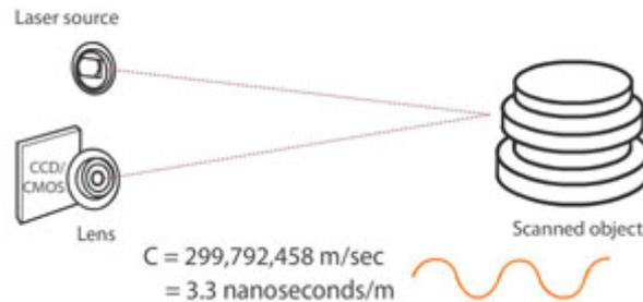
Laser phase-shift systems are another type of time-of-flight 3D scanner technology, and conceptually work similarly to pulse-based systems. In addition to pulsing the laser, these systems also modulate the power of the laser beam, and the scanner compares the phase of the laser being sent out and then returned to the sensor. For reasons that are beyond this web page's scope, phase shift measurement is more precise.
