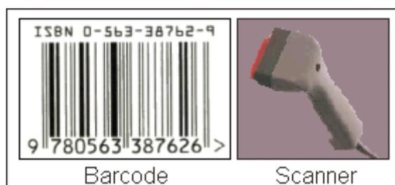
The CCD barcode scanner is a scanner that has no moving parts. **CCD stands for Charged-Coupled Device Scanner**. The scanner has a light source that when pointed to an object or barcode, it illuminates that image. The image is usually a barcode. Once the barcode is illuminated, a reflection is created and the barcode scanner reads that image.
