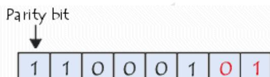
As the parity control system can only detect an odd number of errors, it can only detect 50% of all errors. This error-detection mechanism also has the major downside of being unable to correct the errors it finds (the only way to fix it is to request that the erroneous byte be retransmitted)
