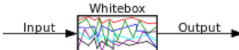
White Box testing model showing various routes through the code being put to test
