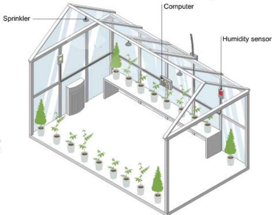
If the temperature falls outside the values stored in the program, the heater is activated by the computer.
