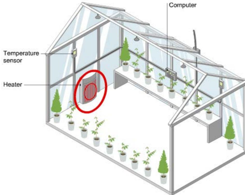
The system monitors the conditions day and night with immediate response to any changes. To alter the growing conditions, the values in the computer program can of course be changed.
